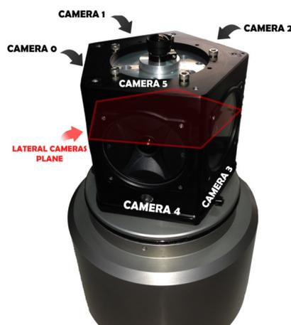
**Figure 3.** Arrangement of the cameras. The red overlay indicates the plane where the optic centers of the five lateral cameras are located (identified as Camera 0 to Camera 4). The last camera (Camera 5) has its optical axis approximately perpendicular to this plane.
