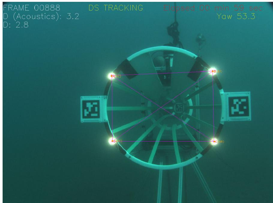
**Figure 5.4:** Debug image of the optical tracking system. In orange the position of the light markers according to the image analysis. In purple, the position of the markers in the DS according to the estimated relative position. AR markers were used as a complementary resource during the final approach when the light beacons were not in the FOV of the camera.
