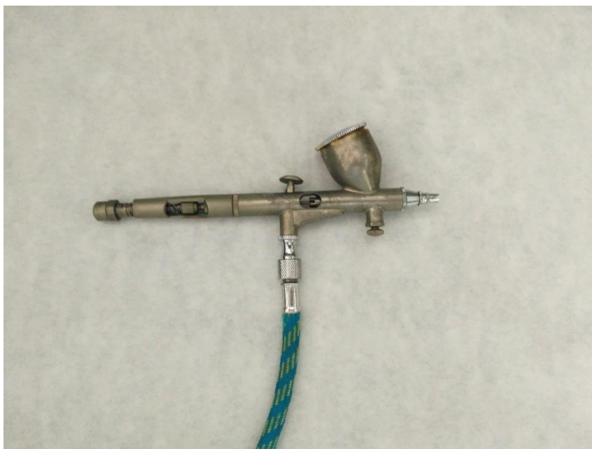
Figure III. 1. Airbrush used for the membrane surface modification.
