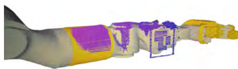
Figure 10. Eight DoF manipulator calibrated. It can be seen how the sensed point cloud overlays the six DoF arm.
