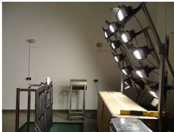
Figure 5.1. Test rig with artificial sun. Lamp array (right) imitating sunlight, with the samples placed opposite. The sample holder consists of a black painted vertical plate (left), on which the pyranometer mounted (white probe) on its upper part
