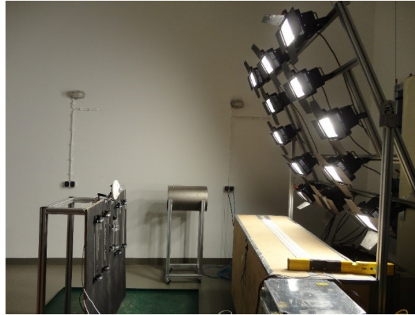
Figure 2.8. Test rig with artificial sun. Lamp array (right) imitating sunlight, with the samples placed opposite. The sample holder consists of a black painted vertical plate (left), on which the pyranometer mounted (white probe) on its upper part
