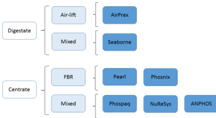
Figure 1.3 Overview of phosphorus recovery technologies from digestate and centrate (adapted from Desmidt et al. (2015) and Kabbe et al. (2015))
