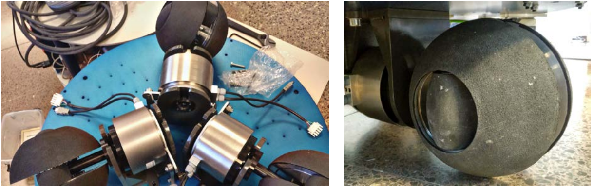
Figure 1.2: Details of the three groups wheel-motor (left) and details of the omni-wheels developed for the mobile base (right).
