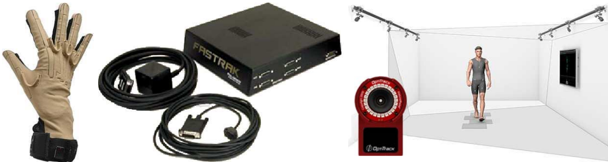
Figure 1.4: Motion-capture devices used in this work: Sensorized gloves (left), magnetic trackers (middle), and optical trackers system (right).
