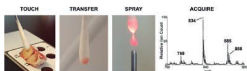
Fig. 1 Swab TS-MS experiment. (Left to right) Tissue is touched with the swab tip and transferred by rotating the swab on its shaft. The swab is positioned in front of a mass spectrometer and an electrospray is generated directly from the swab tip upon application of solvent and a high voltage, which allows mass spectra to be recorded.
