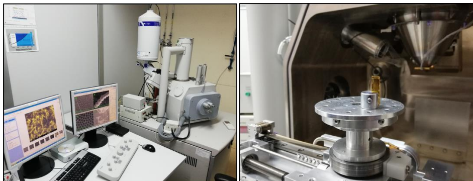
Figure 2.8. ESEM microscope used to analyse fillers and cured samples.
