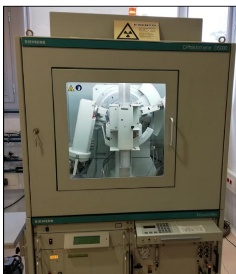
Figure 2.9. Diffractometer Siemens D5000 used in this thesis.
