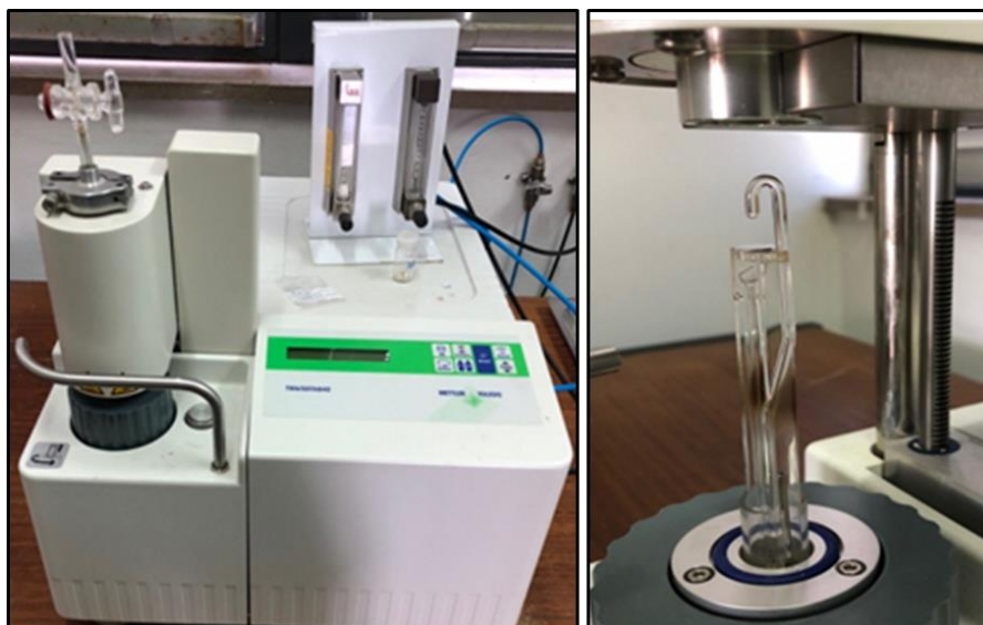
Figure 2.4. Image of TMA device and the probe which subject the sample inside the furnace.
