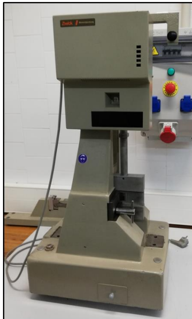
Figure 2.7. Zwick 5110 impact tester used to determine the impact energy absorbed.
