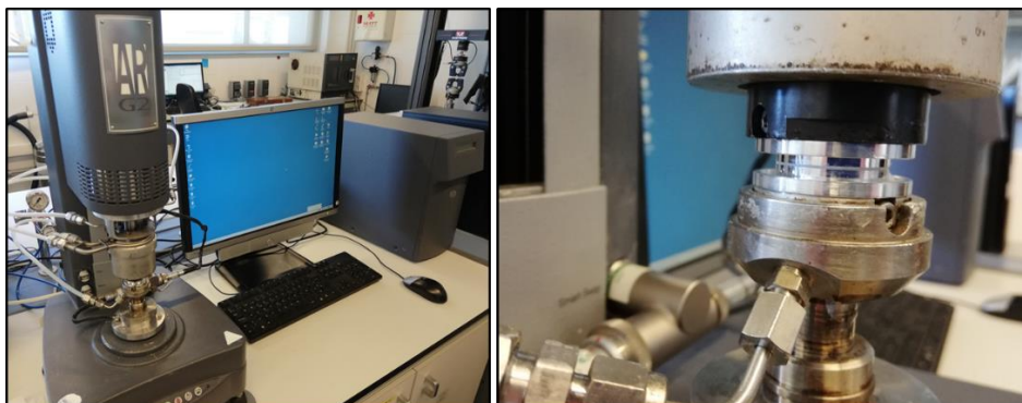
Figure 2.2. AR G2 rheometer from TA instruments equipped with a Peltier temperature controller system.
