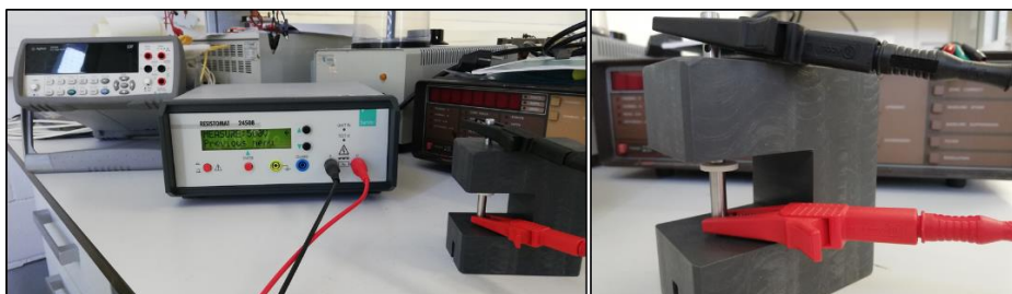
Figure 2.10. The multimeters from Agilent Technologies and Resistomat and a detailed view of the montage to measure the electrical resistance of samples between two electrodes.
