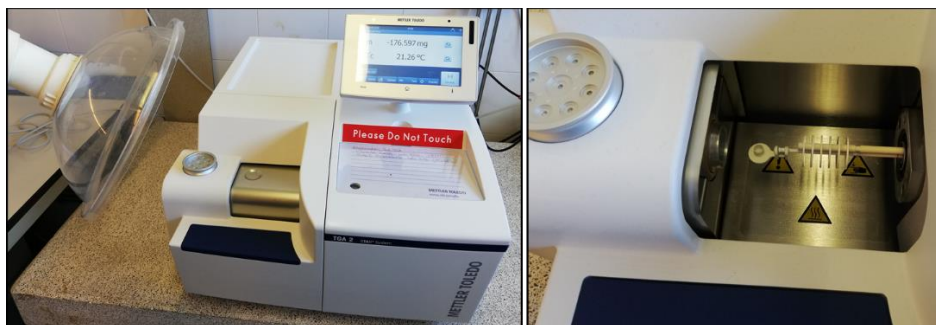
Figure 2.5. Thermobalance Mettler TGA2 and a detailed image of the oven and balance.
