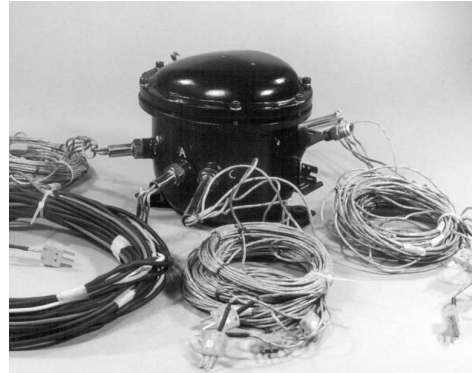
Figure 3.3: Compressor view including thermocouples group.
