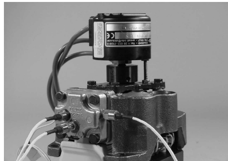
Figure 3.12: Detailed crankcase instrumentation.
