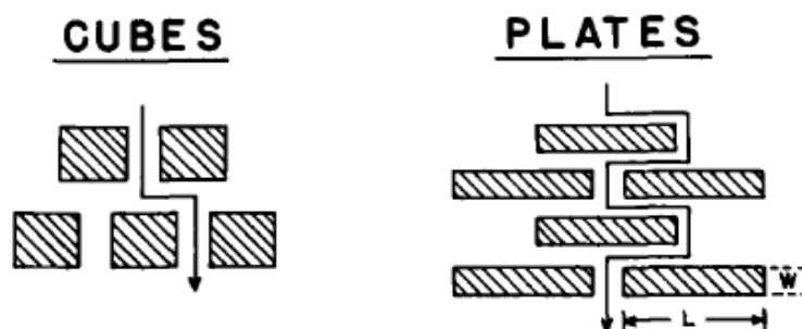
Figure 1.9 Simple model for the path of a diffusing moiety through a filled polymer
