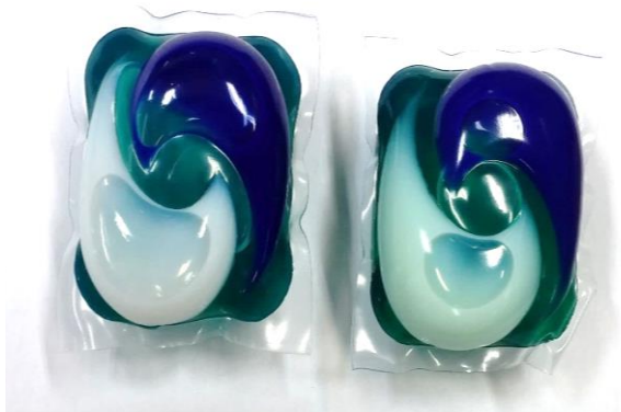
Picture 1.1 Fresh pouch (left) vs aged one (right)
