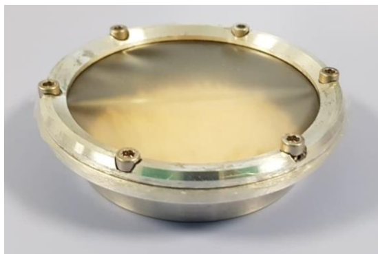
Picture 2.7 Specimen for WVP experiment; film covers the desiccant
