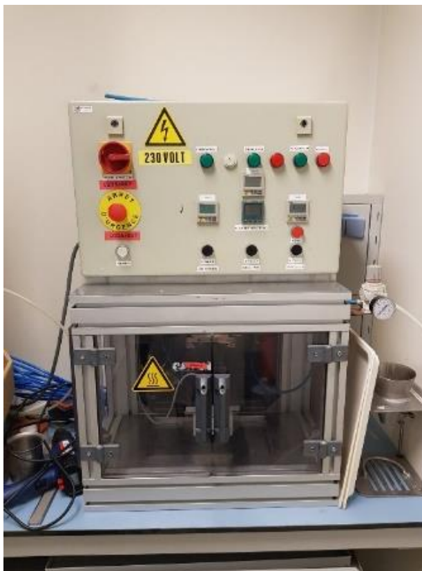
Picture 2.11 Thermo/vacuum machine used for producing a single pouch
