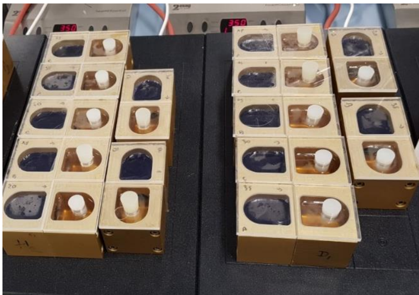
Picture 2.9 Migration experiment cells on hot-stirring plate
