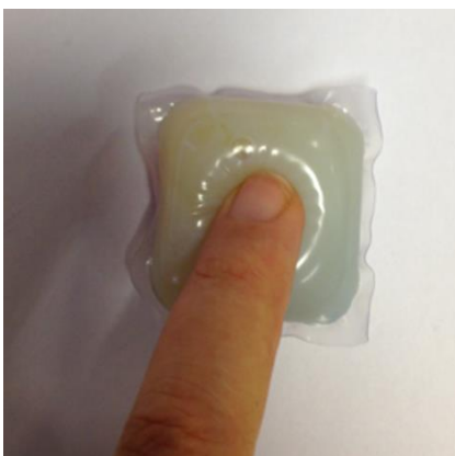
Picture 1.2 Softness due to film permeability
