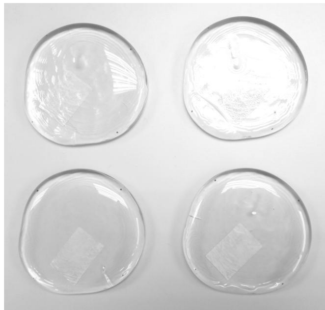
Figure 3. Glass samples obtained from the experimental gob drop tests. Two samples loaded in the side sections on the left and two more loaded in IS3 on the right.
