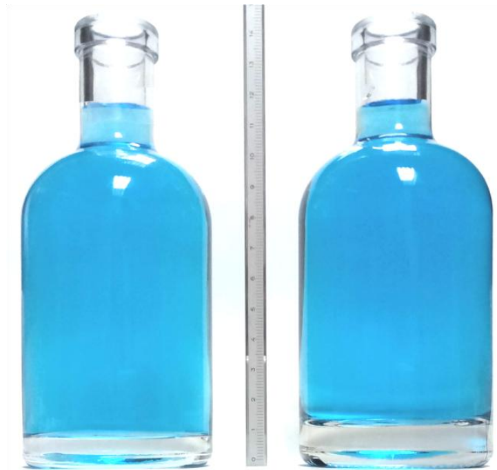
Figure 7. Comparison of the two ALFA 200 bottles manufactured with both blank molds. A lighter container was obtained with blank mold cavity A (left) and a thicker bottom resulted from blank mold cavity B (right).
