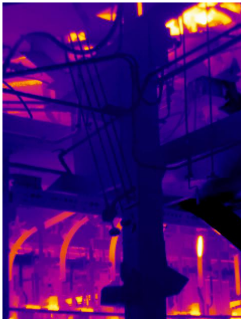
Figure 13. An infrared shot of the IS machine viewed from the blank side using the low-temperature calibration. The glass gobs traveling through the delivery equipment and the amount of time spent in that operation can be determined.
