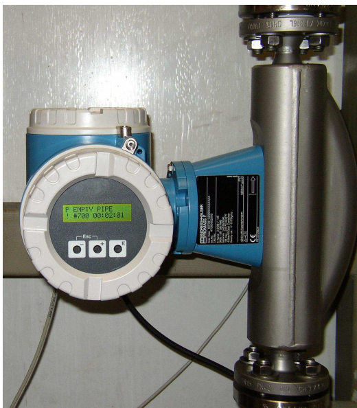
Figure 3.23: Vapour refrigerant mass flow-meter
