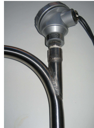
Figure 3.20: RTD Pt100 mounting in a bend
