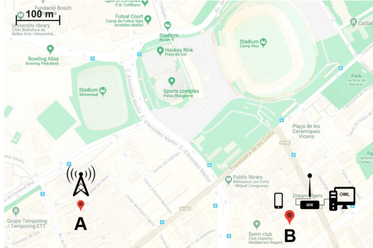
Figure 6.2: Map of Barcelona area where the measurement campaign took place for the creation of the input dataset. The eNodeB location is denoted by A, whereas the data collection system is marked as B.
