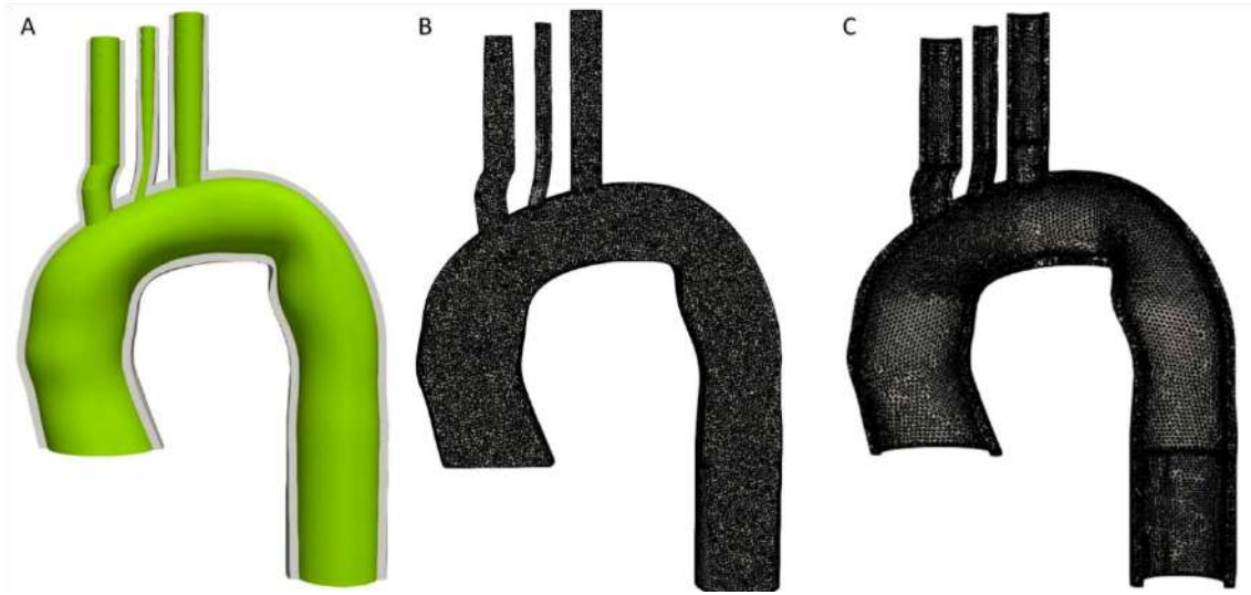
Figure 88. (A) Reconstruction of the aorta vessel and the wall, (B) meshing of the fluid and (C) meshing of the wall.
