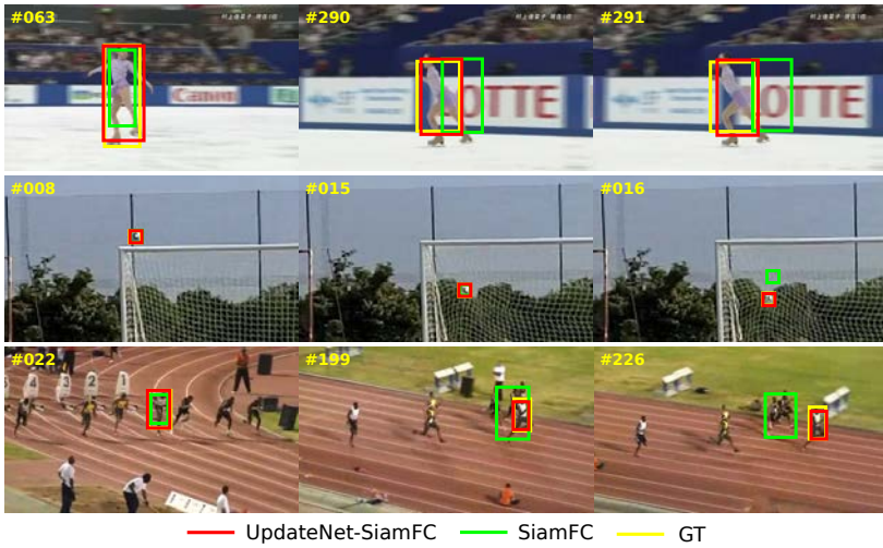
Figure 5.1 – Qualitative comparison between model updates. We learn to update the model template using UpdateNet . When combined with Siamese trackers such as SiamFC (Bertinetto et al., 2016b), our learned updating strategy can be effectively adapted to current circumstances, unlike the simple linear update commonly used.
