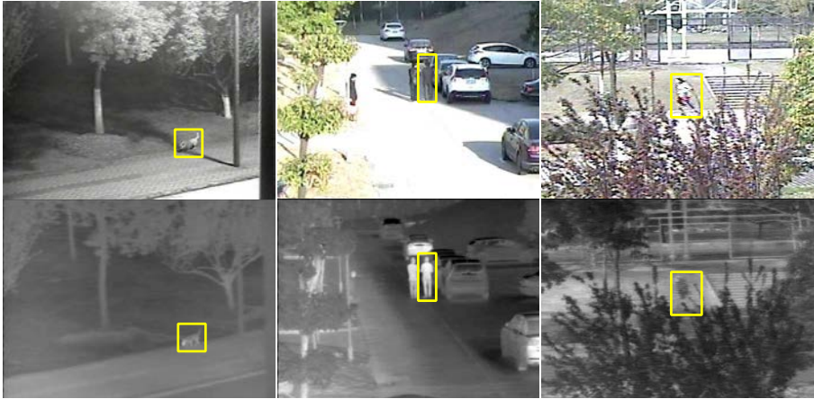
Figure 1.2 – Visualization of the imaging difference between ‘RGB’ and ‘TIR’ for the same scene. On the upper half, we show three exemplar videos from the RGB modality and we show their corresponding videos from TIR modality on the lower half. In the left example, the dog is covered with the shadow from the pole in the RGB modality, but in the TIR modality, this shadow disappears and the target is much clearer than that in RGB modality. In the center example, the human is also discriminative as his temperature is much higher and the shadow from the car disappears in the TIR image. Conversely, the RGB images can also provide complementary benefits over the TIR images. For example, in the right example, the appearance of the person in the TIR image is vague and is heavily influenced by the surrounded tree. While in the RGB modality, the person is clearly distinguished from the surroundings as the color and shape information is very discriminative.
