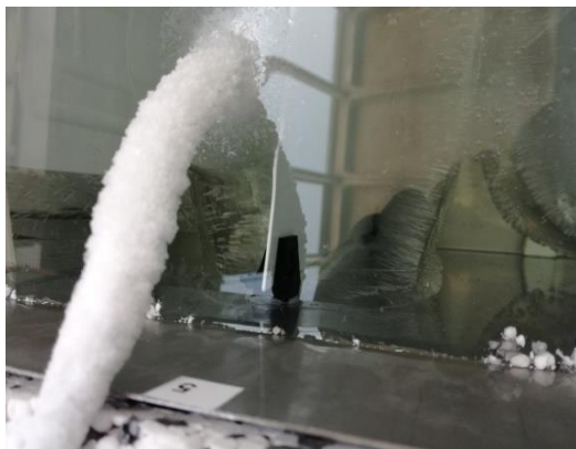
Figure 2. 14 Suction frost observed at evaporator exit and compressor inlet lines for three of the seven scenarios
