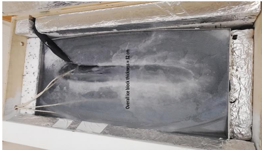
Figure 4. 14 Picture of ice formed showing complete freezing in a 100-litter capacity insulated box and a single modular unit
