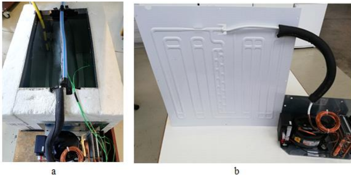
Figure 4. 26 Pictures from experimental campaign (a) Experimental ice storage system developed (b) DC-powered refrigeration cycle unit fabricated
