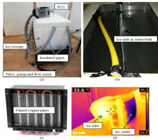
Figure 3. 11 Pictures from the experiment (a) Ice-storage FCU assembly (b) Internal part of ice-storage (c) Internal section of FCU (d) Representative air temperature profile taken by the infrared camera
