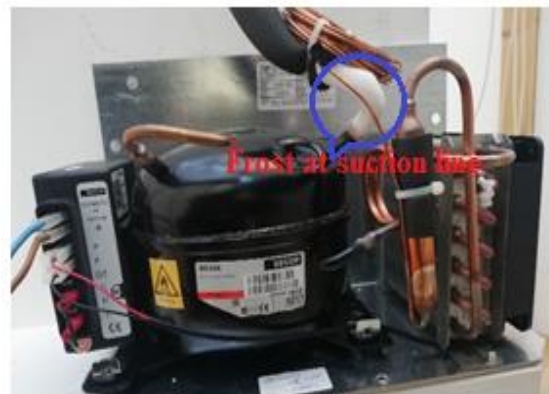
Figure 2. 14 Suction frost observed at evaporator exit and compressor inlet lines for three of the seven scenarios
