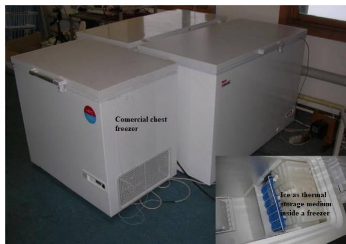
Figure 1. 2 Ice lined freezer for cooling application using PV as energy source [9]
