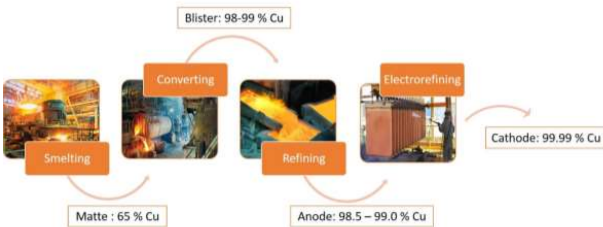
Figure 1. Diagram of conventional copper pyrometallurgical process
