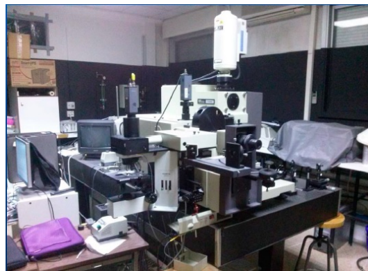
FIGURE 2.1: Jobin-Yvon T-64000 Raman spectrometer at ICMAB-CSIC.
