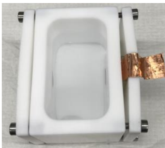
Figure 2.2 Custom designed Teflon box for electrodes to carry out the PEC tests.
