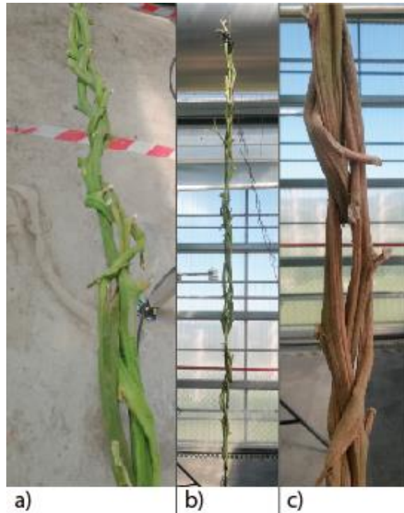
Fig. 42. Braiding and resistance test of tomato stems: a) Braiding process; b) fresh braided stems carrying weight; and c) detail of braided dry stems.
