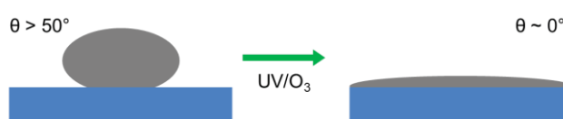
Figure 25. UV/O 3 treatments reduce the contact angle of water to almost zero. It allows excellent wetting behavior of (most) water based precursor solutions on different types of substrates.
