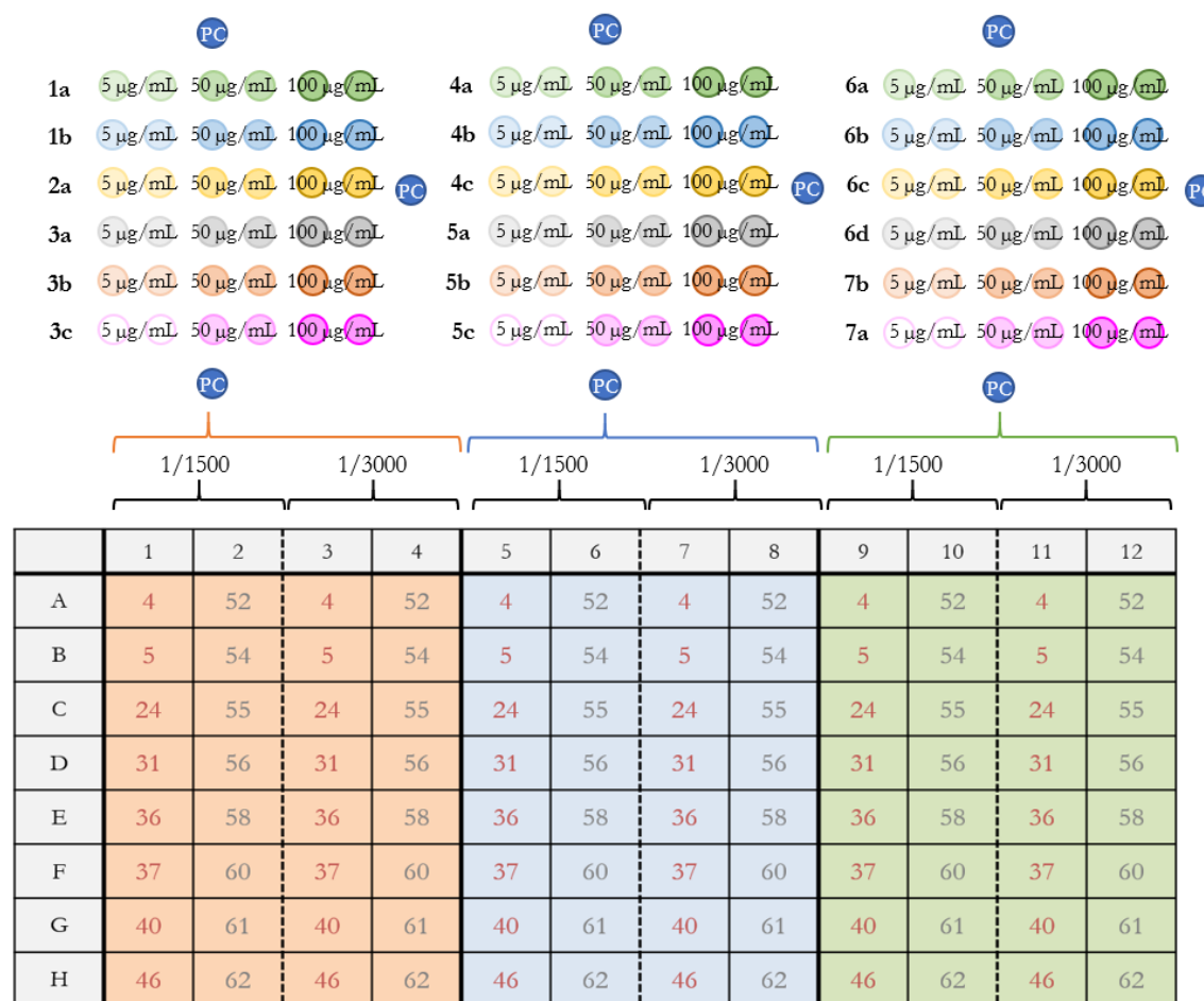
Figure 3-3: Schematic view of the multiplex ELISA (phase I). The upper panel represents the spotting pattern within each section of the 96-well ELISA plate (1 to 3 upper row of the ELISA plate) represented in the lower panel. The first four columns of the ELISA plate were printed with peptides 1a to 3c, Columns 4 to 7 were printed with peptides 4a to 5c, and columns 8 to 12 were printed with peptides 6a to 7b. The eight positive and negative samples were evaluated following the pattern shown in the picture. PC=positive control.
