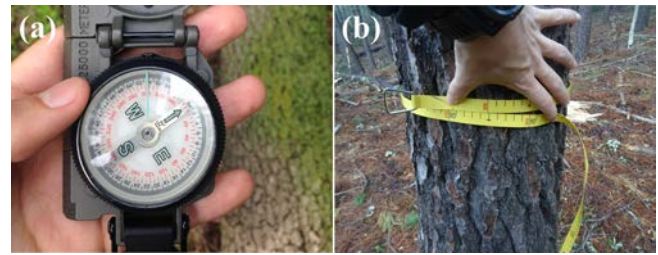
Figure 5. (a) Measure of the fall direction of a tree and (b) measure of trunk diameter during the damage survey of an EF1 tornado on 13 October 2016 in Llinars del Vallès (Catalonia) and an EF2 tornado on 7 January 2018 in Darnius (Catalonia), respectively (author: Oriol Rodríguez).
