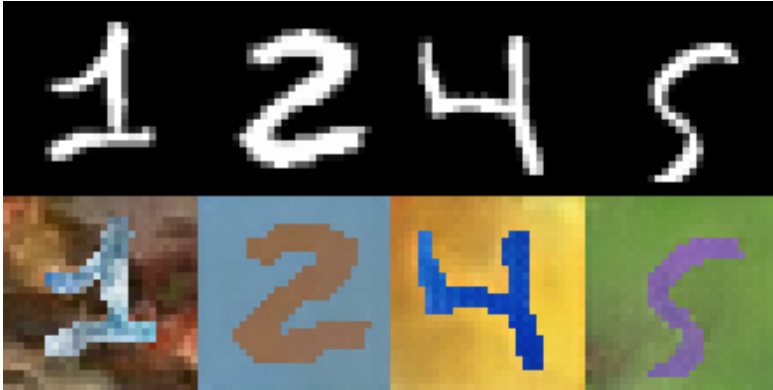
Figure 2.2: A sample from the original MNIST hand written digits dataset in black and white and the extended MNIST-M dataset with different color schemes for the digits and the backgrounds.
