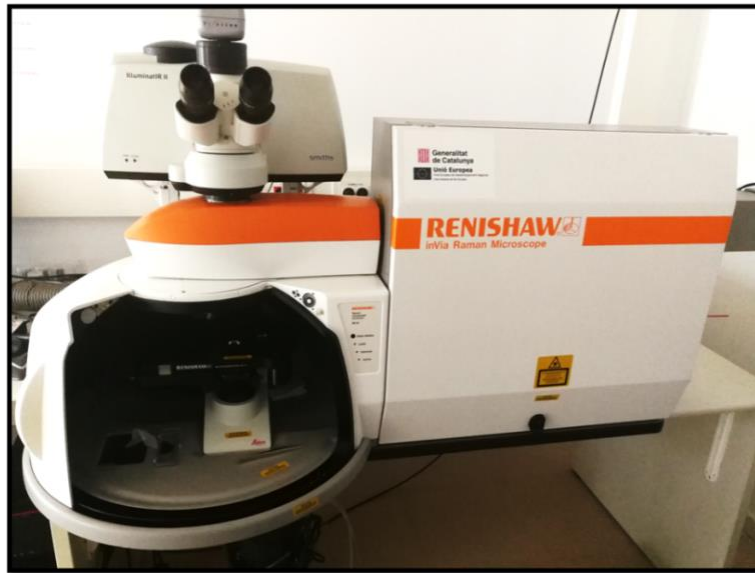
Figure 2-3 Renishaw in Via confocal Raman microscope used in this work for the vibrational characterization of the Tm:Y 2 O 3 transparent ceramic samples
