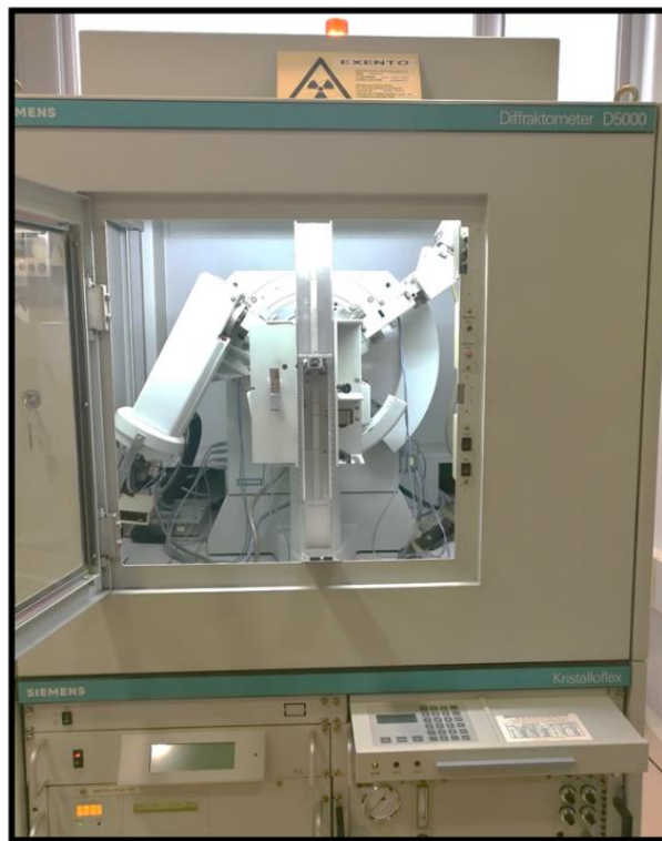
Figure 2-2 Siemens D-500 diffractometer used in this work for the structural characterization of the Tm:Y 2 O 3 transparent ceramic samples.
