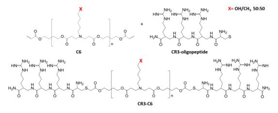
**Figure II-4. Synthesis of the arginine-terminated poly**( $\beta$ -amino ester) C6. Modification of the tri-arginine oligopeptide is shown as an example. Briefly, both the acrylate-terminated C6 polymer and the oligopeptide moiety were dissolved in anhydrous DMSO and mixed at a 1:2.5 ratio (acrylate:oligopeptide). Mixtures remained under magnetic stirring overnight at room temperature and the resultant product was recovered by precipitation.
