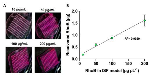
**Figure IV-12. Analyte recovery (RhoB) from mimetic skins with HA-derived MNs.** Increasing intensities in color were observed when sampling ranging concentrations of Rho with the MNs (**A**) Detected RhoB concentration was quantified by absorbance and compared to the real RhoB concentration in HA-based MNs,  $R^2 = 0.9929$  (**B**) Data are represented as mean ± SD (n = 3).
