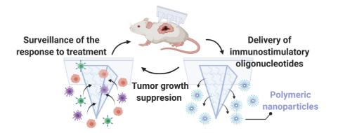
**Figure IV-3. Graphical abstract of Chapter IV.** Throughout this chapter, a new hydrogel-based MN platform has been engineered for transdermal delivery of PBAE-derived polyplexes encapsulating CpG ODNs for cancer treatment while simultaneously surveilling changes in the ISF immune profile as a response to therapy.
