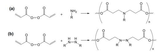
**Figure I-1. Synthetic strategy for PBAEs.**<sup>31</sup> Synthesis of linear PBAEs is achieved by conjugate addition of primary (a) or bis(secondary amines) (b) to diacrylates. Synthesis can be conducted either as a solvent free reaction or in anhydrous organic solvents such as DMSO, chloroform and dichloromethane to avoid hydrolytic degradation.
