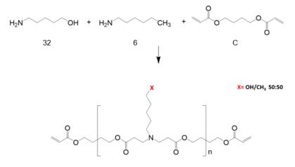
Figure II-3: Synthesis of the acrylate-terminated poly( $\beta$ -amino ester) C6 via Michael addition. Reaction proceeded overnight under magnetic stirring at 90°C maintaining an inert atmosphere. The resulting polymer was precipitated, dissolved in anhydrous DMSO (100 µg/µL) and preserved at -20°C until further use.
