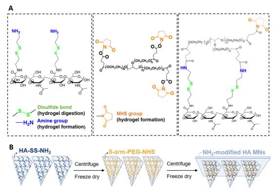
Figure IV-6. Design and fabrication of a novel MN platform using amino-modified HA. Chemical backbone of the HA polymer was engineered to include an amine group (for hydrogel formation) and a disulfide bond (for hydrogel digestion). When reacted with an 8-arm-PEG crosslinker, a highly swellable hydrogel was generated (A). Schematic representation of the fabrication method via successive addition of the two hydrogel components (B).
