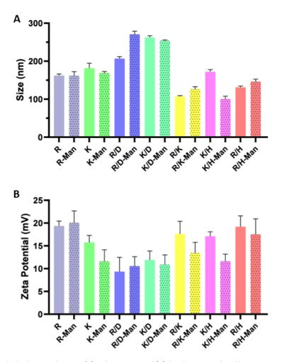
Figure II-7: Average hydrodynamic diameter (A) and zeta-potential (B) distributions analyzed by Dynamic Light Scattering. Polyplexes deriving from the complexation of pDNA with OM-PBAEs and MM-PBAEs were prepared at a 50:1 polymer:pDNA ratio. Polydispersity index (PDI) values were lower than 0.3 for all measurements. Results are shown as mean and standard deviation of triplicates.
