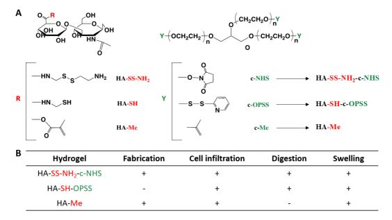
**Figure IV-4. Newly synthesized family of HA-derived MNs for** *in situ* **drug delivery and ISF sampling.** HA was modified via EDC/NHS activation using amino- and thiol- groups or a with methyl methacrylate to generate a library of hydrogel formulations for MN fabrication (A). Candidates were prescreened to identify outperforming formulations for theranostic purposes where [+] indicated a positive readout whereas [-] meant that the hydrogels did not met the needed requirements (B).
