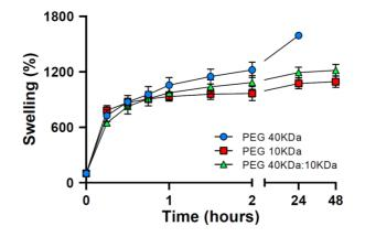
**Figure IV-7. Swelling rate of the HA-based hydrogels composed of amine-modified HA polymer.** The HA polymer was crosslinked with NHS-terminated 8-arm PEG crosslinkers differing in molecular weight. Weight of the hydrogels was recorded as a function of time using PBS as a buffer mimicking ISF. Data are represented as mean ± SD (n = 3).
