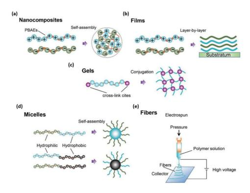
**Figure I-2. Schematic representation of PBAE-derived systems.**<sup>48</sup> Thanks to their chemical flexibility, PBAEs can be formulated using different approaches in accordance with their final application. Nanocomposites (polyplexes), films and micelles have been extensively described for drug delivery, yet others such as gels or fibers are of particular interest for tissue engineering.
