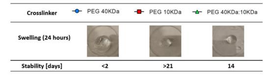
**Figure IV-8. Hydrogel disks stability when incubated in physiological-relevant conditions.** Hydrogels were incubated in PBS at 37°C under gently rotation and monitored daily.
