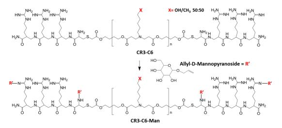
Figure II-5 Synthesis of mannose-modified PBAEs from OM-C6 polymers. Decoration of the arginine-modified PBAE is shown as an example. OM-PBAEs were dissolved in anhydrous DMSO with allyl- $\alpha$ -D-Mannopyranoside (ADM). Reactions were allowed to proceed overnight at room temperature under stirring and resulting polymers were precipitated with a mixture of diethyl ether and acetone (70:30 v/v). Red R's indicate the most provable site of reaction.
