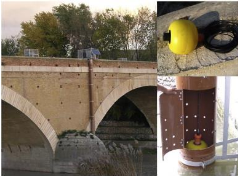
Figure 3.4. Upstream view of Carapelle cross section, gauge station and probe housing device.
