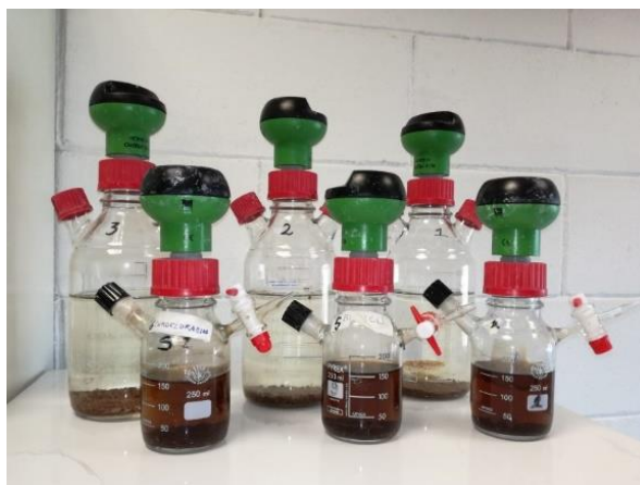
Figure 4.5 First inhibition test: front-line bottles, tannery WW test during phase 4; back-line bottles, control test.
