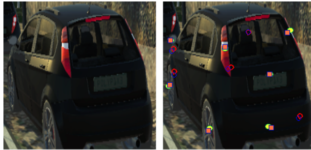
Figure 3.14: Predicted 2D keypoints on synthetic vehicle extracted from virtual KITTI dataset.
