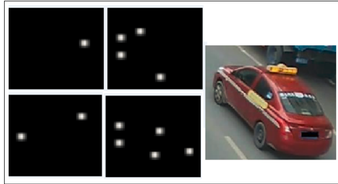
Figure 3.10: Predicted heatmaps with gaussian drawn around detected keypoints extracted during training and validation phase.
