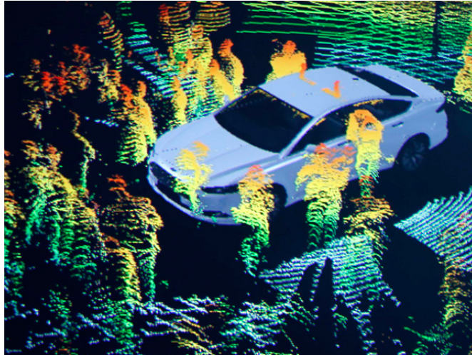
Figure 2.2: Illustration of the measurement of a LIDAR sensor [4].
