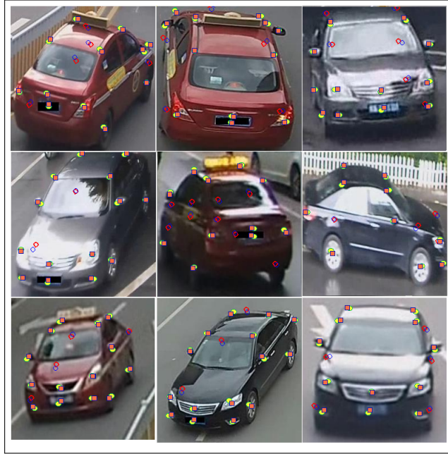
Figure 3.11: Results of keypoint detection vs. ground truth labeling considering also self-occluded points in the vehicle. The yellow circles are the predictions and the red squares mark the ground-truth with non-occluded points. Blue circles are ground truth and red circles are predictions of keypoint position with self-occluded points (partially or totally occluded).
