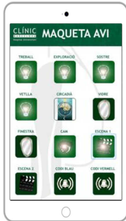
Figure 20. GUI of the building automation system. The function “Treball” corresponds to support lighting; “Exploració” corresponds to medical examination lighting; “Sostre” corresponds to ceiling lighting; “Vetlla” corresponds to floor lighting; “Circadià” corresponds to circadian lighting; “Vidre” corresponds to the state of polarization of the door; “Finestra” corresponds to the state of polarization of the windows; “CAM” corresponds to the state of video streaming from the camera (on/off); “Escena 1” corresponds to “Scenario 1”; “Escena 2” corresponds to “Scenario 2”; “Codi Blue” corresponds to a code blue; and “Codi Vermell” corresponds to a code red.
