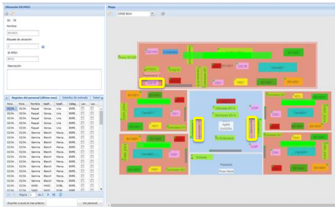
Figure 66. The Infobox web application with the RTLS software and the location of the electronic dispensers highlighted in yellow.
