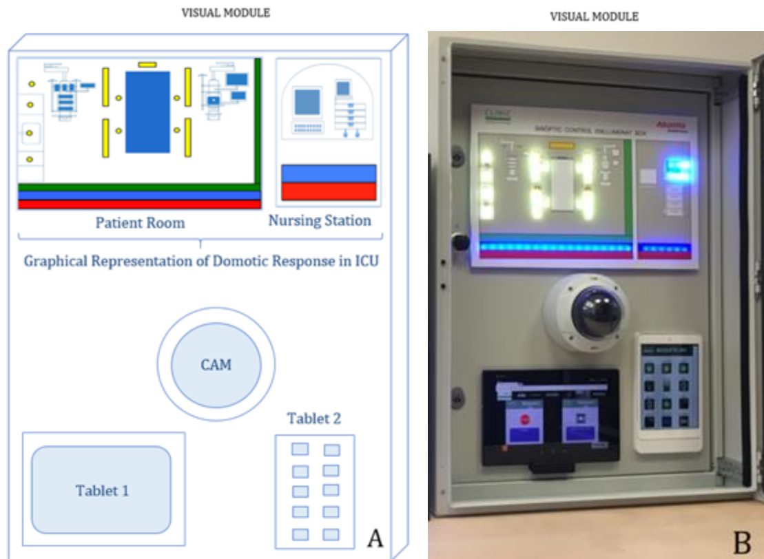
Figure 18. Visual module of the prototype used to simulate automated responses in the room and nursing station of the ICU. On the left side, there is the sketch and the right side there is the resulting manufacturing physical prototype of this module with all its elements highlighted. CAM: camera; ICU: Intensive Care Unit.
