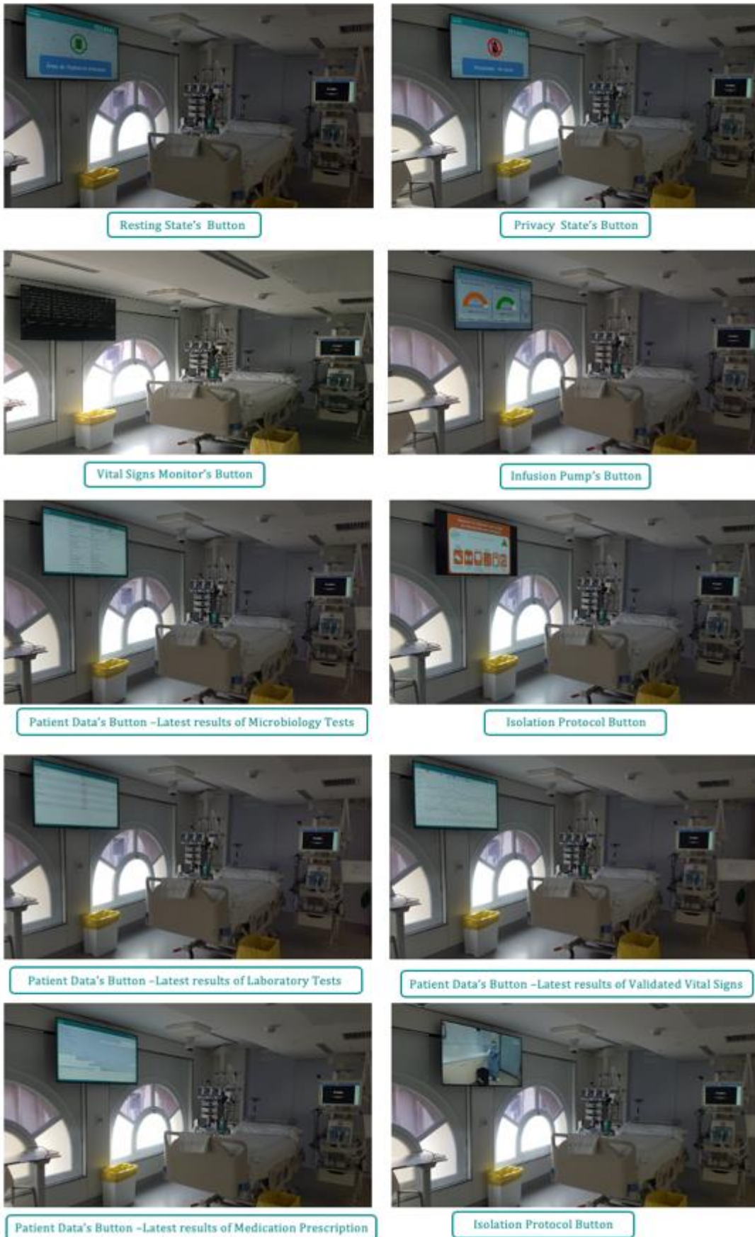
Figure 54. Examples of the layouts that the clinical resources control interface can display on the screen in a patient room.
