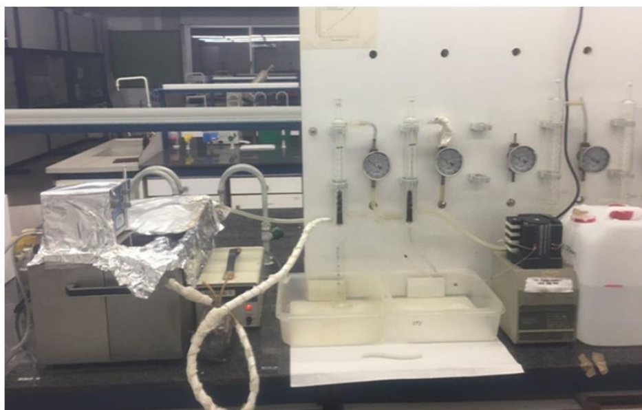
Figure 6.2. Experimental set-up of a the fixed-bed column with water bath used for arsenic adsorption.
