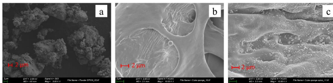
Figure 3.4. SEM images of SPION(a), sponge (b) and sponge-loaded SPION (c).
