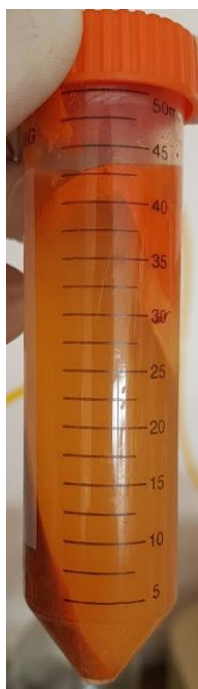
Figure 1. Vial of SBJ after centrifugation. Upper part of the vial: oil juice phase, middle part of the vial: clarified SBJ, lower part of the vial: rests of seeds and peel and pulp.
