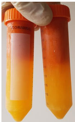
Figure 14. Phase separation of non-filtered SBJ after 24h of freezing with the styrofoam jacket (as it is schematically represented in Figure 5).
