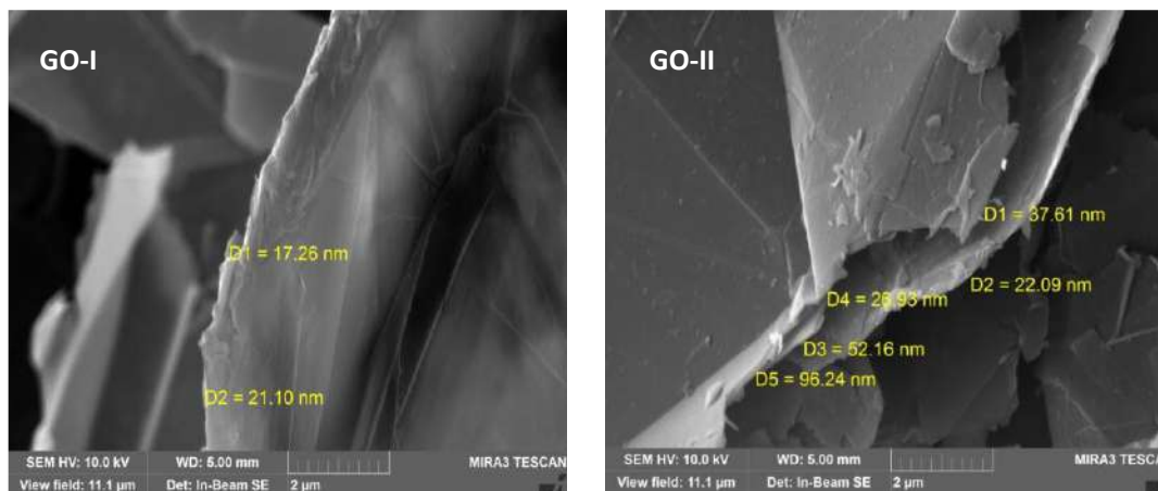
Figure 4.30. SEM image at 50.000 x showing the thickness and surface of graphitic oxides plates of GO-I and GO-II and plate size homogeneity (Ševčík, 2020).
