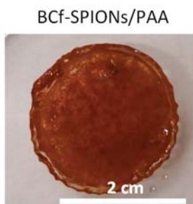
Figure 13: Photocurable BCf/PAA hydrogel with BCf decorated with SPIONs obtained after 2 min of UV irradiation.
