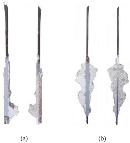
Figure 7.9. (a) S3-B-PSL-225-10-30 failure in the A-C interface; (b) S3-B-PSL-225-7.5-30 cohesive failure in the concrete.
