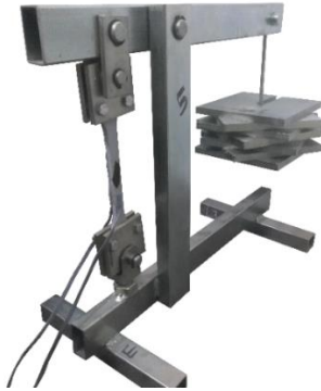
Figure 5.4: Experimental test set-up of the adhesive characterization under sustained loading.
