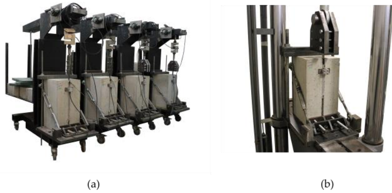
Figure 7.2: Set-up used for (a) SL tests; (b) PSL tests.
