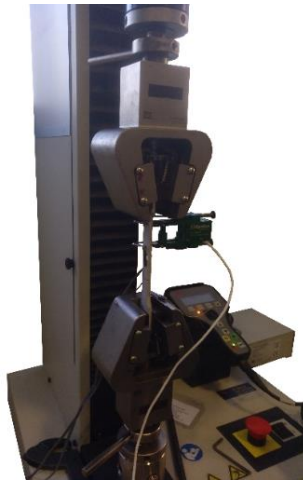
Figure 6.1: Set-up for the instantaneous tensile test of adhesive specimens.
