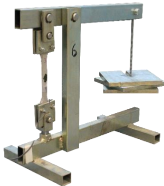
Figure 6.3: Set-up of the sustained loading test.
