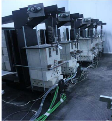
Figure 2.17: Experimental set-up for tests under sustained load used in Emara et al. [73].
