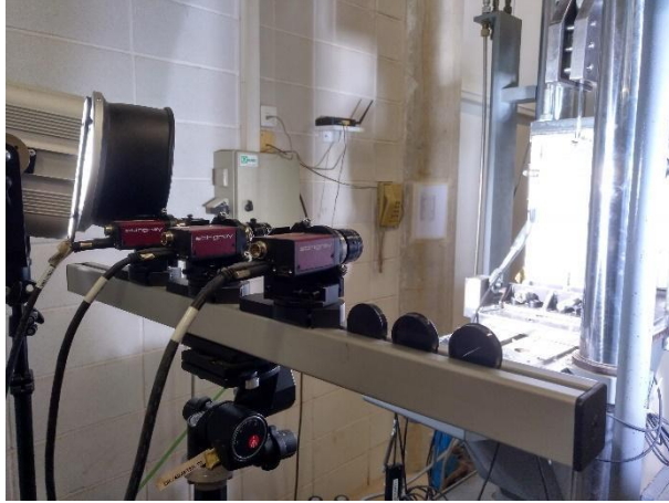
Figure 3.8: DIC system installed in the instantaneous test.
