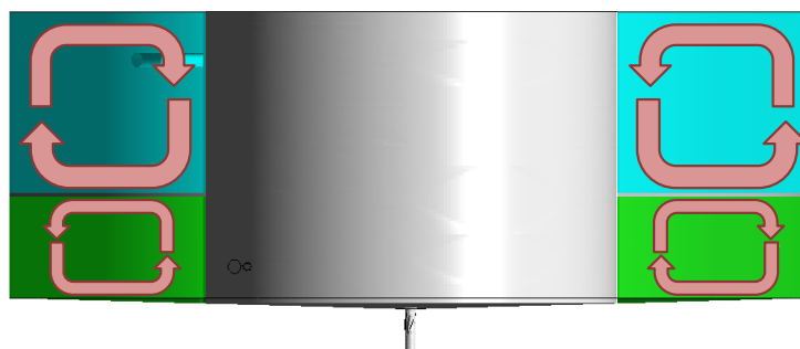
Figure 3.8: Upwards and downwards secondary flows in DYNOMIX and Turbulent Flow regions.
