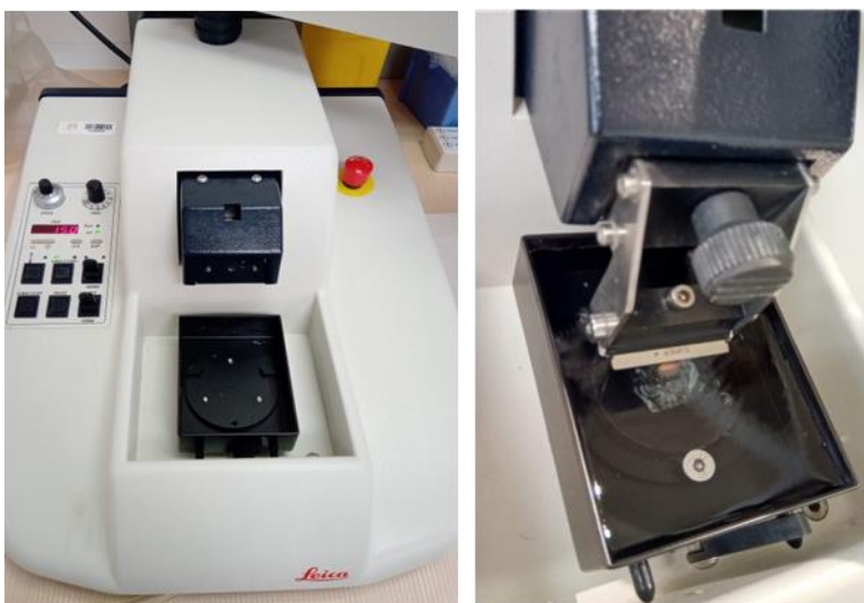
Figure 3: Vibratome (leica) used for wheat grain sectioning (right), sample mounted in glycerol bath (left).
