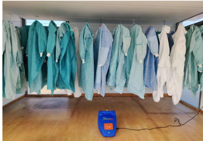
Figure 18 Automated disinfection method decontaminating different PPE in a Spanish Hospital.
