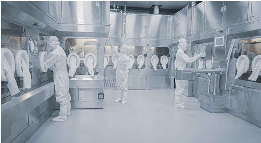
Figure 10 Aseptic process of filling and loading unloading process to a freeze dryer. Facility manufactured by Azbil Telstar Technologies. A line of isolators together with an automatic loading and unloading system is introduced.
