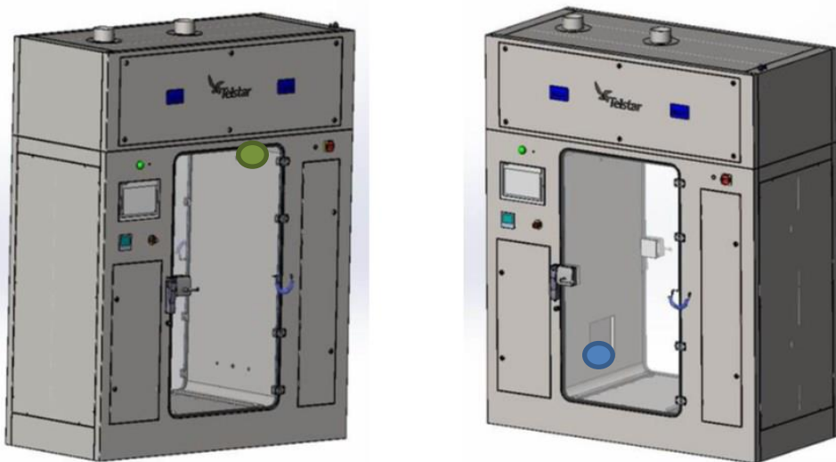
Figure 52 Passthrough box for Computational Fluid Dynamics (CFD) simulation: Relief (green circle) and nozzle (blue circle)
