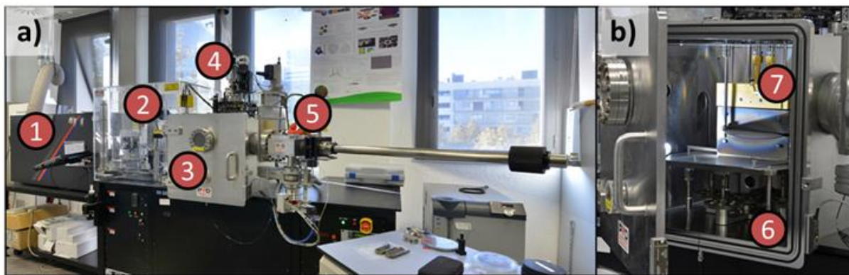
Figure 2.2. a) Picture of the PLD equipment installed at IREC and b) detail of the vacuum chamber (number 3 in Figure 2.2-a)
