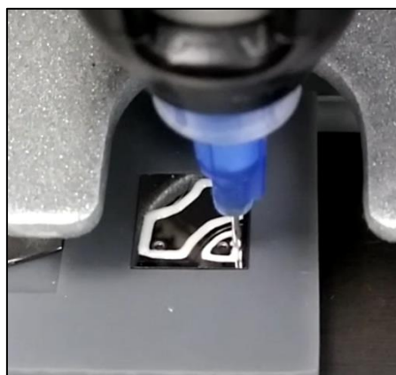
Figure A.9. Optical image representing the extrusion of the slurry from a nozzle (robocasting)
