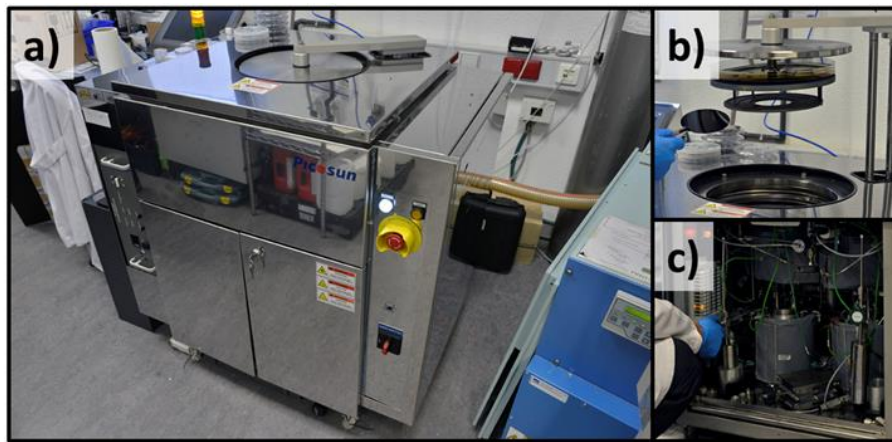
Figure 2.5. Optical image of a) industrial ALD system from PicoSun used in this work, b) the wafer holder and reactor chamber and c) cylinders and gas lines for the precursors.
