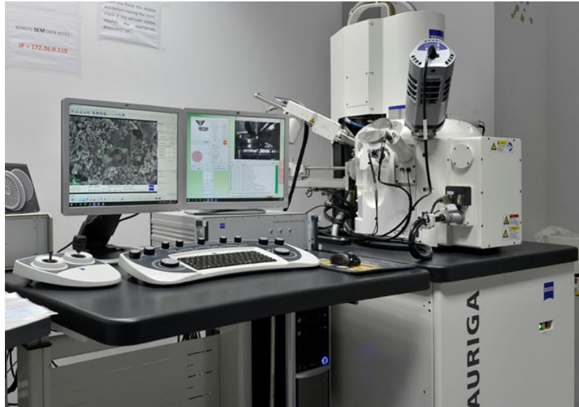
Figure 2.14. Scanning Electron Microscope AURIGA from Zeiss, located at IREC
