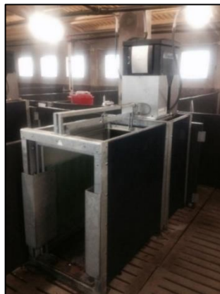
Figure 8.1. Automatic feeding system (Nedap ProSense®, The Netherlands) used in the studies presented in the present PhD dissertation.
