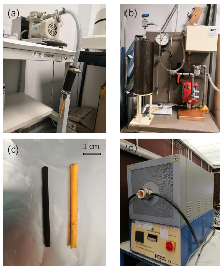
Figure 7.1. Procedures of the preparation of the polycrystalline \text{YBaCuFe}_{0.95}\text{Mn}_{0.05}\text{O}_5 rod: (a) the powder was packed with cylindrical shape using the vacuum bump; (b) the powder was further packed with the isostatic press; (c) the resulting packed rod with cylindrical shape after the previous procedures; (d) the furnace used to perform the sintering/annealing process for the rod.
