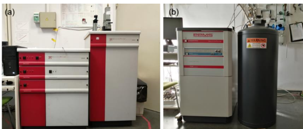
Figure 2.4. The (a) SQUID and (b) PPMS magnetometer located at the Low Temperature and Magnetometry Service Lab in ICMAB.
