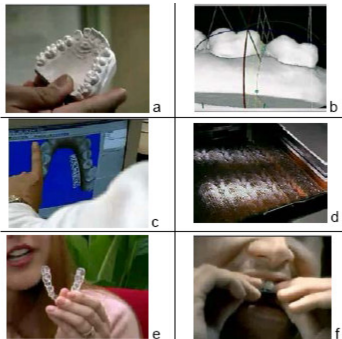
Figure 2.15 Individual set manufacturing process chain for each patient: a) dental impression, b) digitised data elaboration, c) STL forming tool data, d) tooling sets on SLA 7000 system, e) thermoformed biocompatible transparent plastic bridge, f) bridge use in mouth (Levy 2003)
