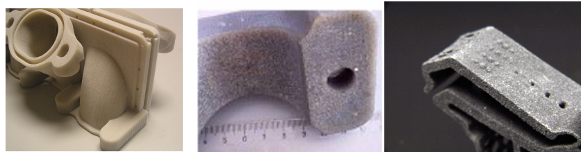
Figure 3.10 Surface finish for some RM processes: Left to right: SLS PA, SLS on Duraform Flex, and MJM
