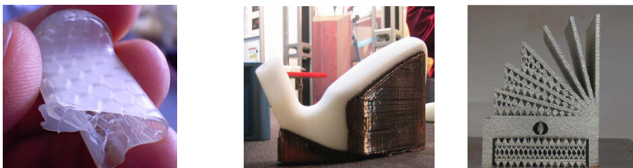
Figure 3.124 Some support structure types for RM. Left to right: SLA Quickcast, FDM Water soluble support, SLM with stainless steel
