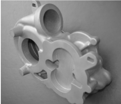
Figure 2. 13 A water-pump built by the SLM process(Vilaro, Abed et al. 2007)
