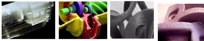
Figure 3.113 Stair-stepping appearance for some technologies: From left to right SLA, 3DP, inkjet, MJM
