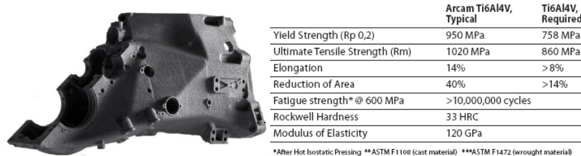
Figure 8. 2 Gear Box manufactured with Arcam RBM in Ti6Al4V and the properties claimed by the manufacturer source ( http://www.arcam.com )
