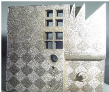
Figure 8. 4 Benchmark part produced on a SLM concept Laser and material specification for Stainless Steel 17-4. Source (Katholieke Universiteit Leuven 2008)
