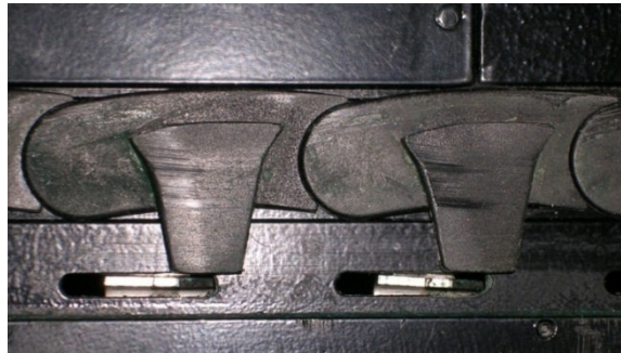
Figure 9. 43 Image of the moving “links” with wear marks due to continuous movement inside the machine and contact with coins
