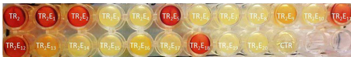
Figure S9. Visualization of the transaminase activity assays of the purified TR 2 mutants (reaction: 8 h) using hexanal as the substrate.
