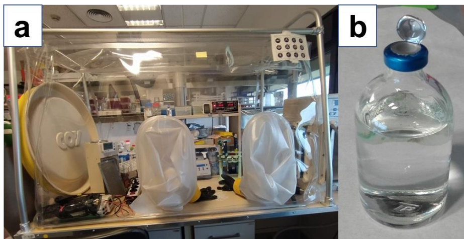
Figure 3.3. Anaerobic glovebox used to prepare the anaerobic medium (Panel A) and glass serum bottles with anaerobic medium (Panel B).
