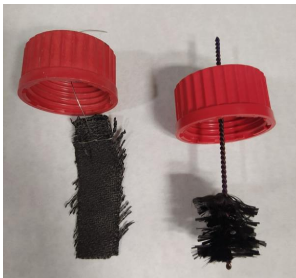
Figure 5.2. Carbon cloth (left) and graphite fiber brush (right) electrodes used in the cathode of the experimental BES.
