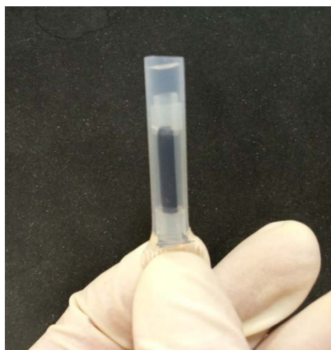
Figure S1. Experimental set-up used for the preparation of molded polymeric monoliths in PTFE coated magnets.
