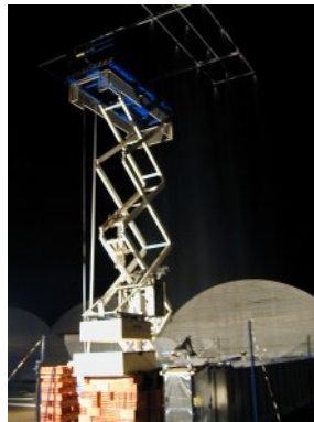
Figure 5.15. Rain generator mounted at 13 m.
