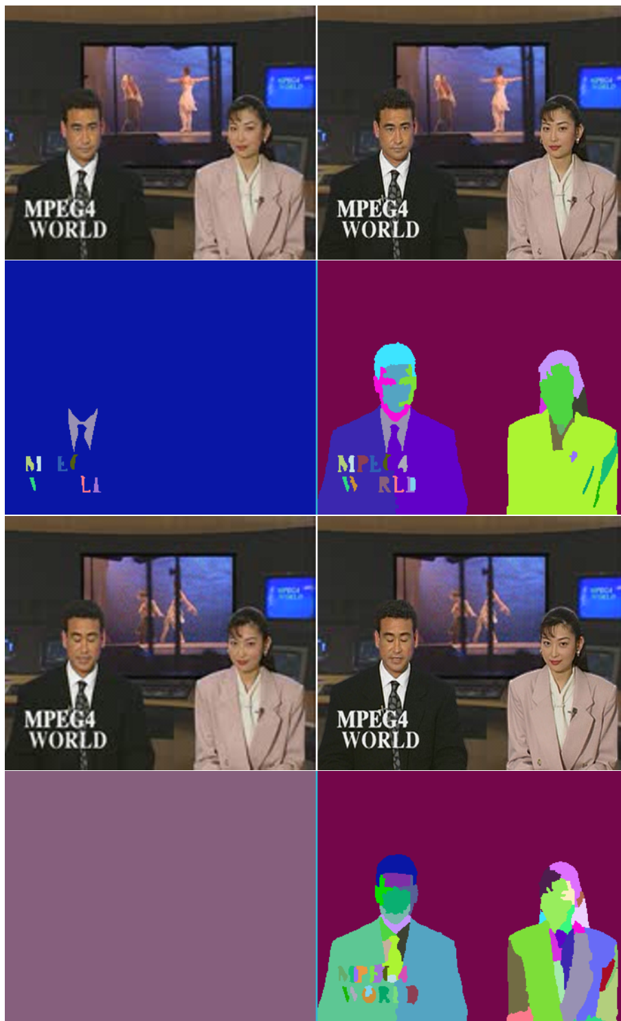
Figure 9.19: Example of Spatial scalability: News sequence (CIF) coded at 10Hz, object functionalities mode, 128 kbps (base layer, QCIF) + 384 kbps (enhancement layer, CIF). Figure shows base (up-sampled by a factor two) and enhancement layers in the first row and the corresponding partitions in the second row for frames #0 and #60
