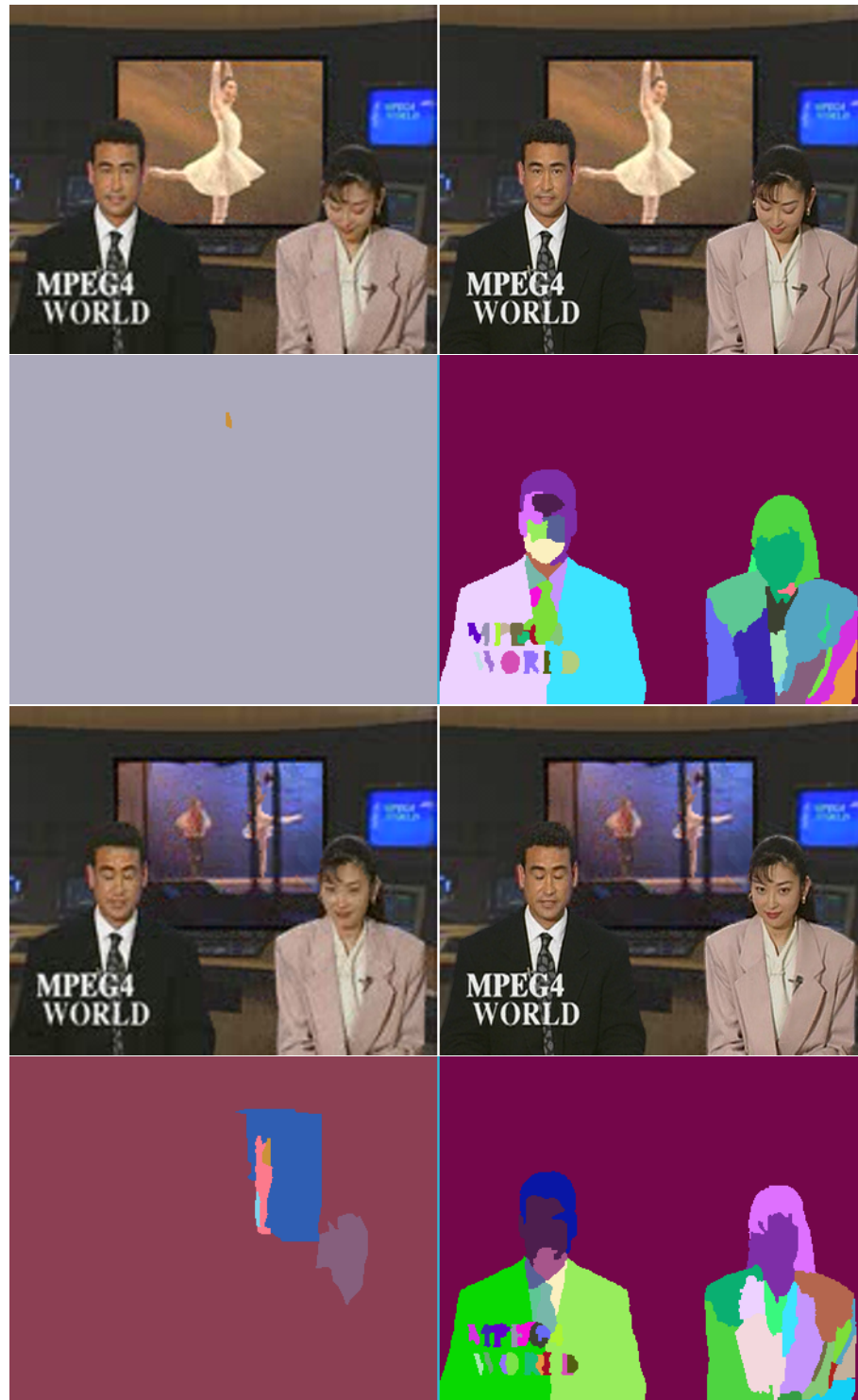
Figure 9.20: Example of Spatial scalability: News sequence (CIF) coded at 10Hz, object functionalities mode, 128 kbps (base layer, QCIF) + 384 kbps (enhancement layer, CIF). Figure shows base (up-sampled by a factor two) and enhancement layers in the first row and the corresponding partitions in the second row for frames #120 and #180
