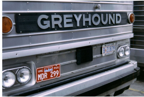
Figure 1.1: 24 GHz VORAD radar mounted at the front side of a Greyhound bus [5]
