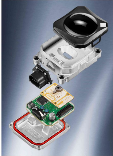
Figure 1.3: Exploded view of the Bosch LRR3 sensor [9]
