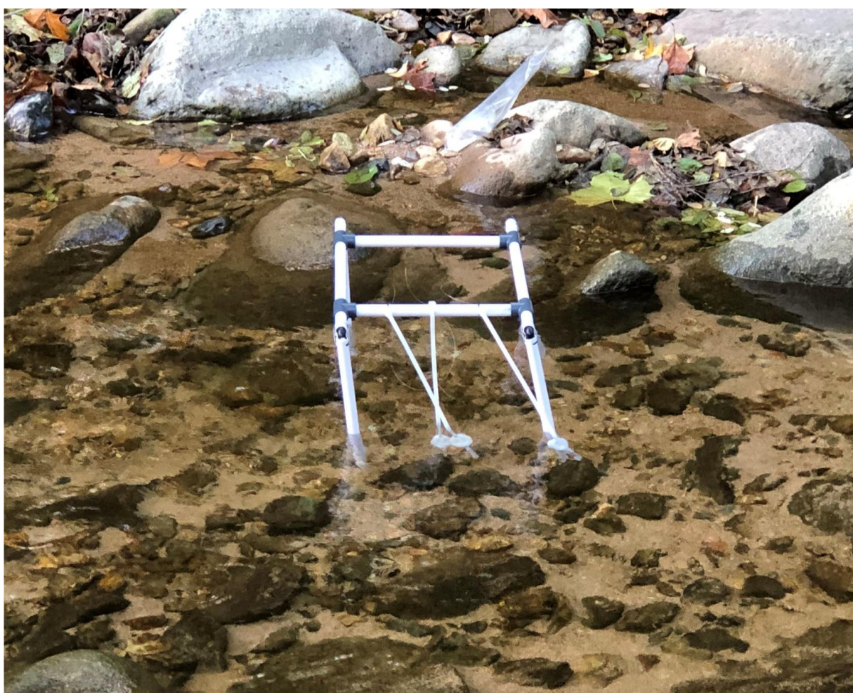
Figure 7.1 Parallelepiped structure holding DGT devices parallel to the river flow to sample Osor stream.
